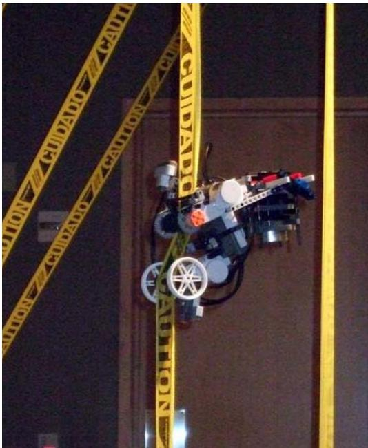
Figure 21. Model climber on the tether with the center of mass off to one side of the ribbon. The climber is distorting the ribbon to put the center of mass directly under it.
